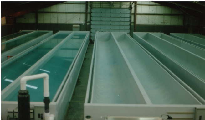
Figure 14: Cross-flow tanks for the sea bass nursery
