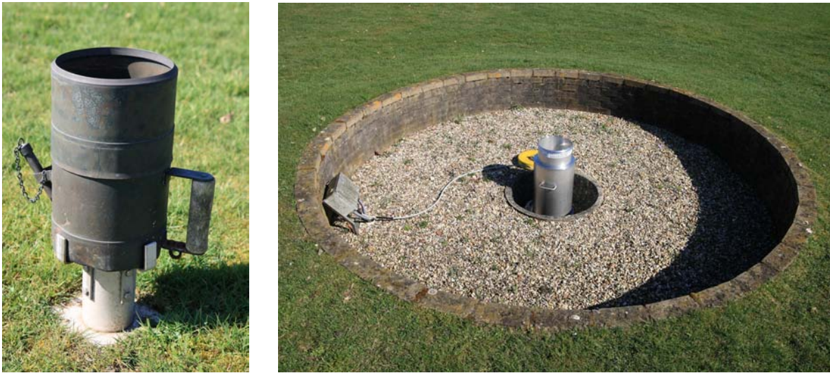
Figure 1.4: The manual rain gauge (left) and the automatic rain gauge (right) part of KNMI's rain gauge networks.
