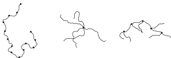
Figure 1.2: Linear, star, and comb polymer architectures. Beads on the linear chain mark the length of statistical segment.
