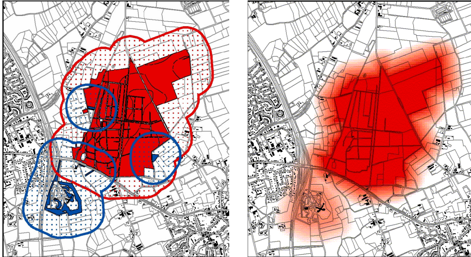
Figure 1: Transition areas based on crisp buffer (left) and on fuzzy buffers (right).
