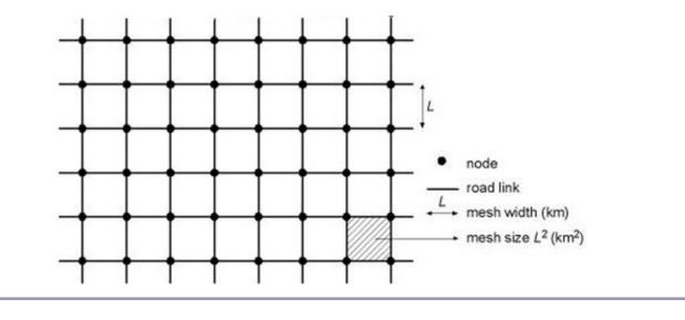
**Fig. 1.** Schematic representation of a network of minor roads in a regular square grid. The grid has nodes and road links with a length of *L* kilometres.
