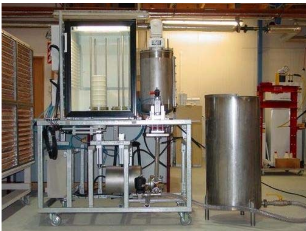
Figuur 11 Protein fractionation robot (PFR) (Chand, 2006)
