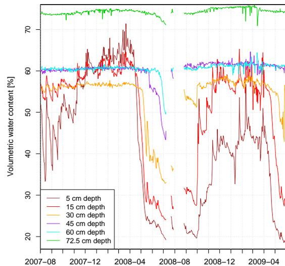
Figure 3. Volumetric water content, averages over 6 sensors at the same depth.
