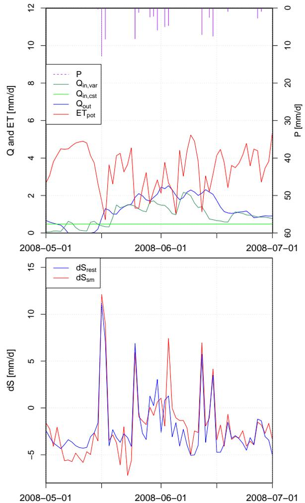
Figure 5. Daily sums of water balance terms for a summer period for the whole catchment (top) and storage change computed as rest term and from soil moisture data (bottom).
