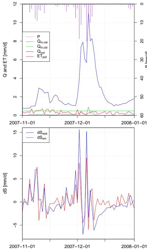
Figure 4. Daily sums of water balance terms for a winter period for the whole catchment (top) and storage change computed as rest term and from soil moisture data (bottom).
