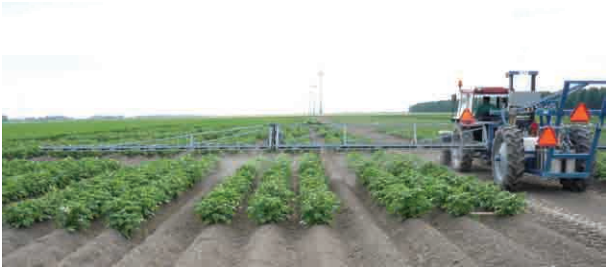
Photo 1: One of the beams of the Sosef-trial-spraying machine (in another experiment). Every time the spraying machine goes to the experimental field 10 different products can be sprayed.
