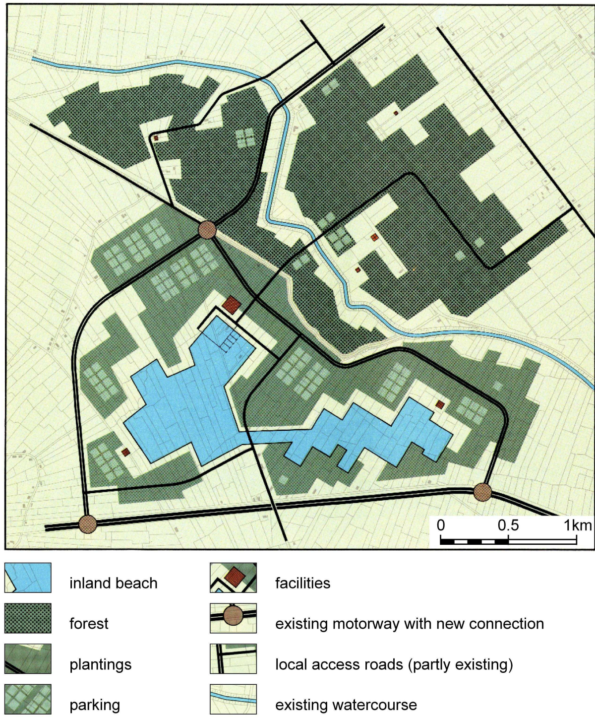
Figure 1. Design in the late 1960s for a “green star” development in the countryside, with an area of about 10 km 2 and a planned capacity for 75,000 recreants, with 65,000 of them traveling a distance of 15 km or more (Dorschkamp & Stiboka, 1971)
