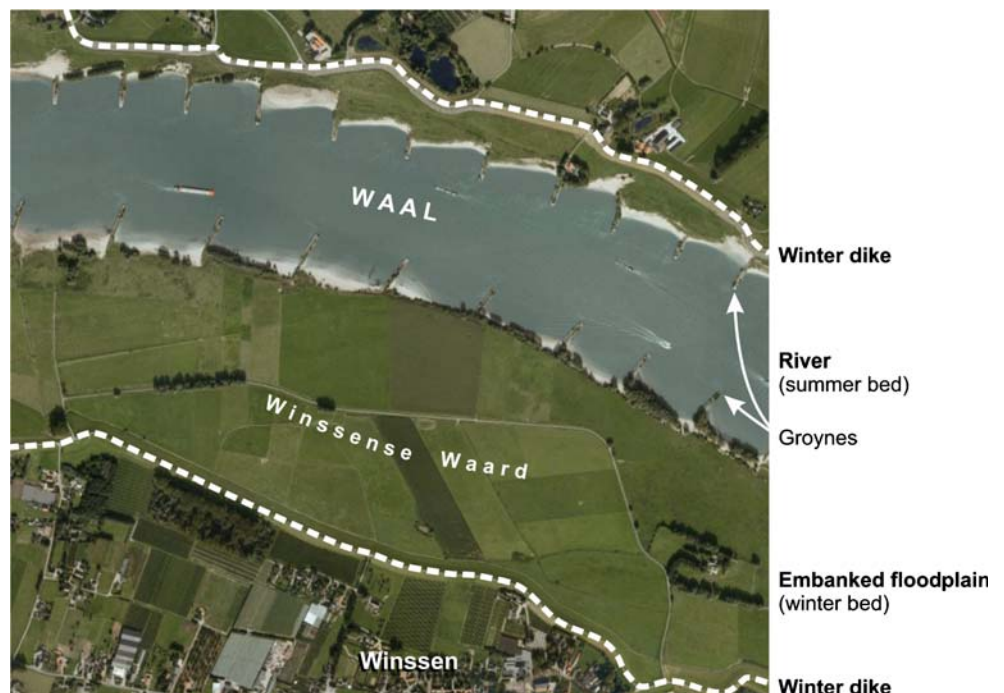
Fig. 4 Aerial photograph of the Winssense Waard, an embanked floodplain along the Waal distributary of the Rhine (see Fig. 1 for location)
