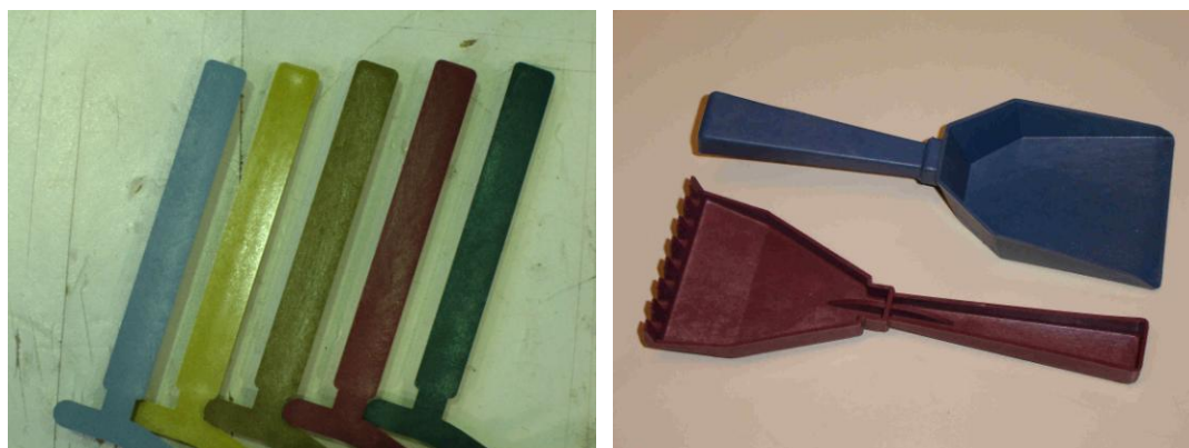
Figure-12: Flexural test bars with 25% of jute fibre and household items with 40% of jute fibre, all containing 2% of pigment.
