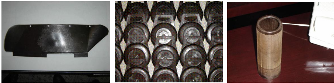
Figure-14: Products made from 40 wt.% Jute-PP after adequate drying: Back plate of magazine cover (left), Electric cable cover (middle) & Bobbin (right).
