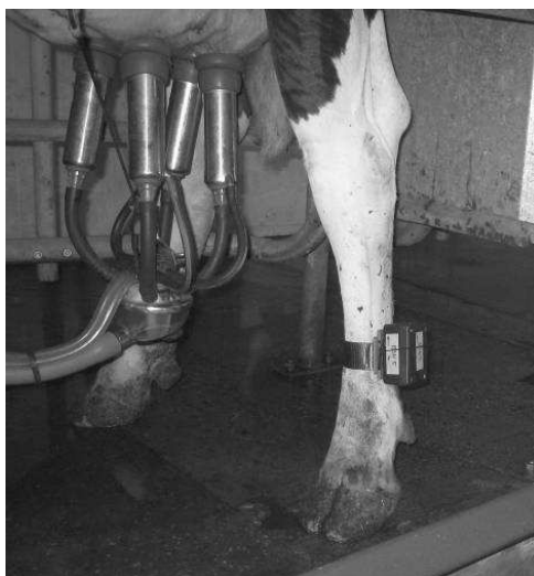
Figure 2. Attachment of a node to the left hind leg (picture taken during milking).
