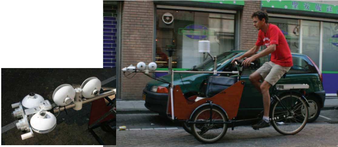
Fig. 2: Mobile biometeorological station mounted on a cargo bicycle
