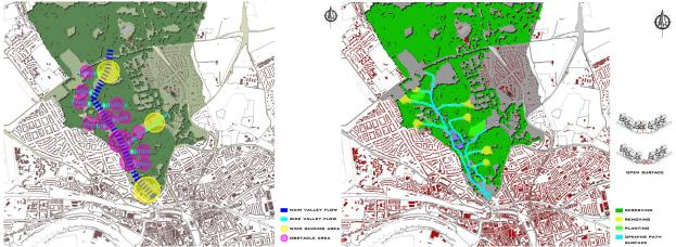
Figure 9 (left) analysis of expected cold air generation and flow paths and obstruction areas and Figure 10 (right) redesign proposal for the whole park for optimal cold air production and passage
