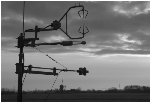
Fig 2.6. Eddy covariance measurements in the field. (licor 7500 Irga with a Campbell Scientific Csat Sonic anemometer and standard meteorological equipment; according To the CarboEurope protocol)
