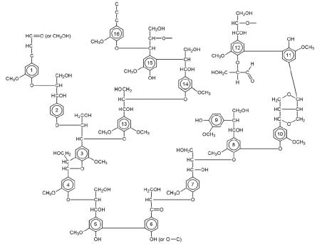
Figure 6 Model structure of spruce lignin
