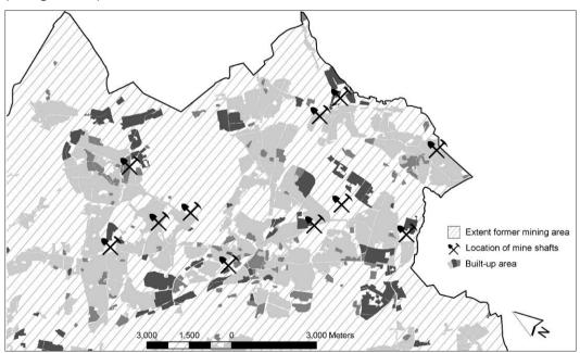
Figure 3-10. Map of the Parkstad region (The Netherlands). Potential for the vertical stratification of energy systems by means of heat (cold) storage in former coal mines.
