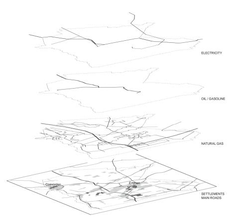
Figure 6-6. Different energy subsystems in the region of Southeast Drenthe.
