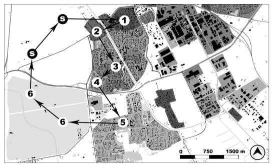
**Figure 3-3.** Proposed heat cascade in Emmen-Noordbarge (The Netherlands). Residual heat from gas processing units (S) is transported to the oldest neighbourhood (1) and further through more recent neighbourhoods with lower heat demand (2 - 5), to planned neighbourhoods with lowest heat demand (6).
