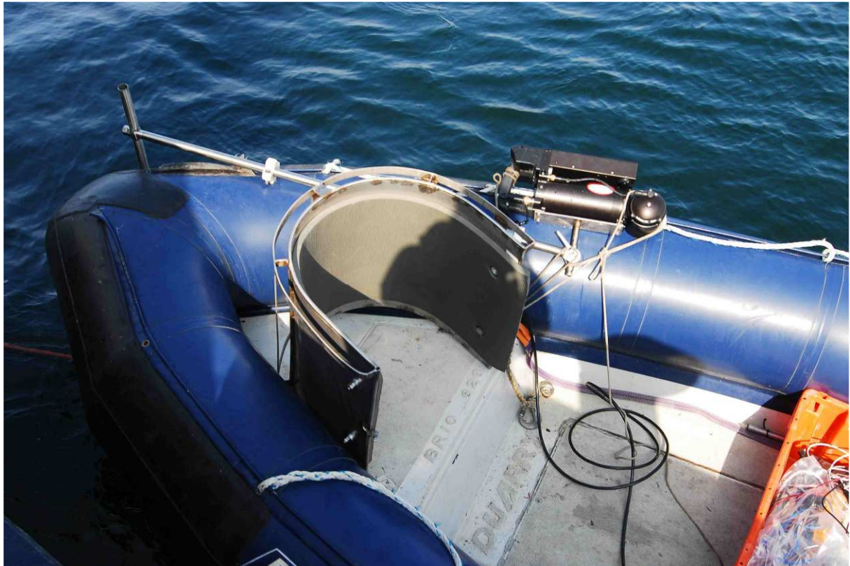
Photo 4. Deployment device to operate the DIDSON at the transects from an inflatable boat.
