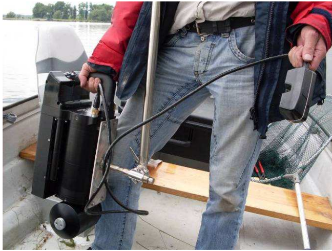
Photo 1. DIDSON as stand alone unit with the diving mask.
