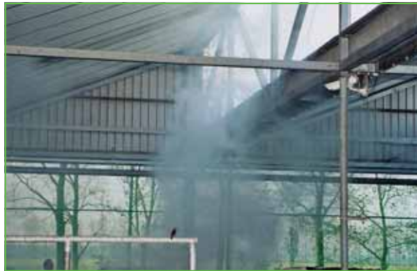
Picture 6. Test with artificial smoke to check the amount of ventilation and the pattern of the air flow
