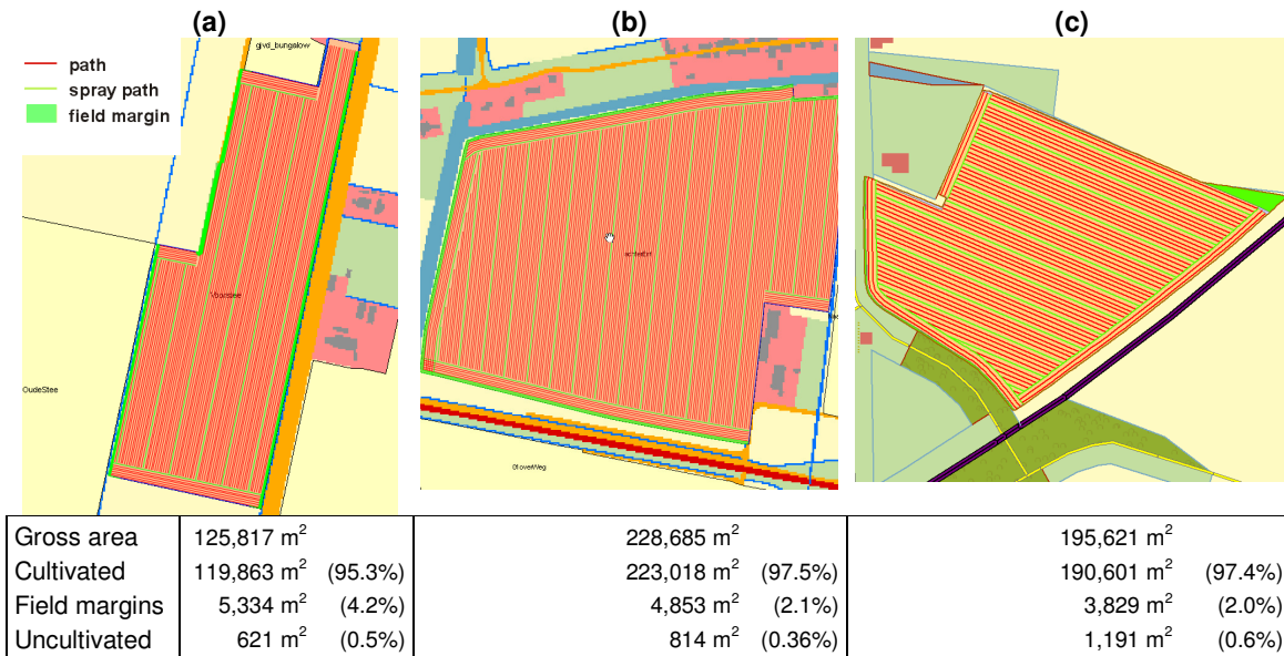
Fig. 5. Example results obtained from GAOS (a,b) and manual editing in a GIS (c).
