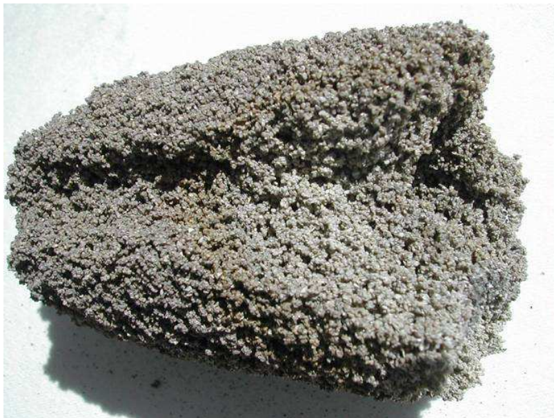
Figure: Bed agglomerate removed from a fluidized bed combustor burning a blend of 10% rice straw in wood fuel after 3.5 h of operation (courtesy Prof Bryan Jenkins, University of California)
