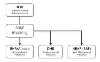
Figure 1: Processing scheme for reflectance products
