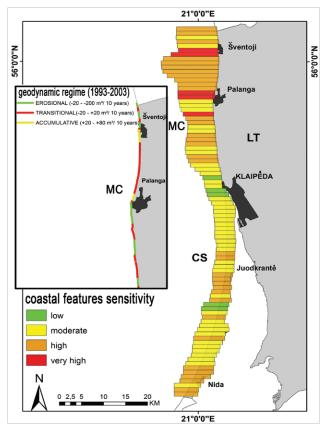
Fig. 3. Representation of the coastal features sensitivity and a detailed view of erosion and accumulation processes (sand volume refers to 1 m of coast line) between Palanga and Šventoji. Compiled by D. Depellegrin, 2010.
