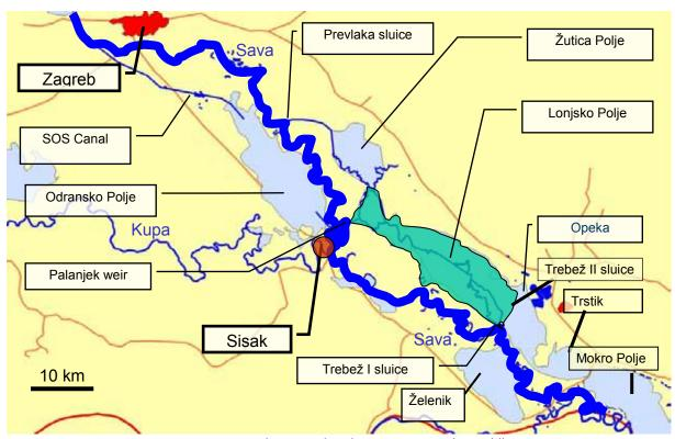
Figure 4. Retention areas plus in- and outlet structures in the Middle Sava area
