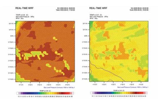
Modelled spatial distributions of air temperature at 2m, Sea Level Pressure (hPa), and wind velocity at 10 m for 5 August 2003, 17:00 (left panel) and 19:00 UTC (right panel).
