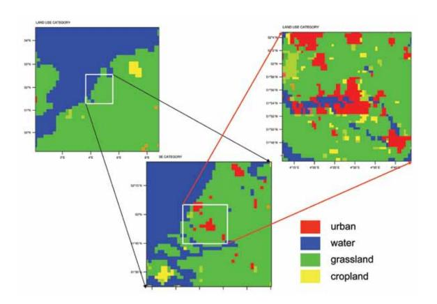
The three domains used for the land use configurations, with the city of Rotterdam in the centre (51,9167 N; 4.4667 E). Resolution domain 1: 25 x 25 km ( $41 \times 41$  grid cells). Resolution domain 2: 5 x 5 km ( $41 \times 41$  grid cells). Resolution domain 3: 1 x 1 km ( $61 \times 61$  grid cells).
