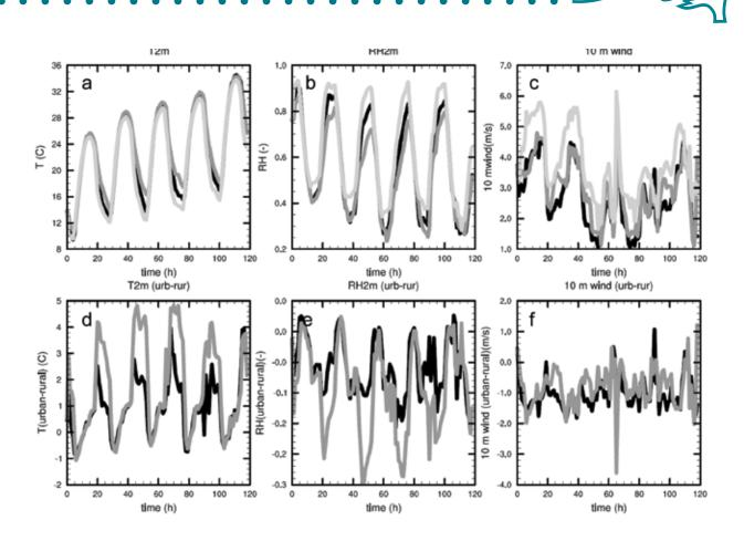
Modelled air temperature (a) and relative humidity (b) at a height of 2 m, wind speed at a height of 10 m (c), differences in air temperature (d), relative humidity (e) and wind velocity (f) between the urban and rural area, 15-20 July (start model simulation: 15 July 00:00 UTC). Black line: Rotterdam north (51 °56'; 4 °30'). Dark grey line: Rotterdam south (51 °53'; 4 °31'). Light grey line: rural area (51 °58'; 4 °40').
