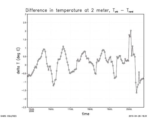
The calculated differences in simulated air temperature at 2 m between a grid cell in the city of Rotterdam and a grid cell 30 km northwest of Rotterdam .
