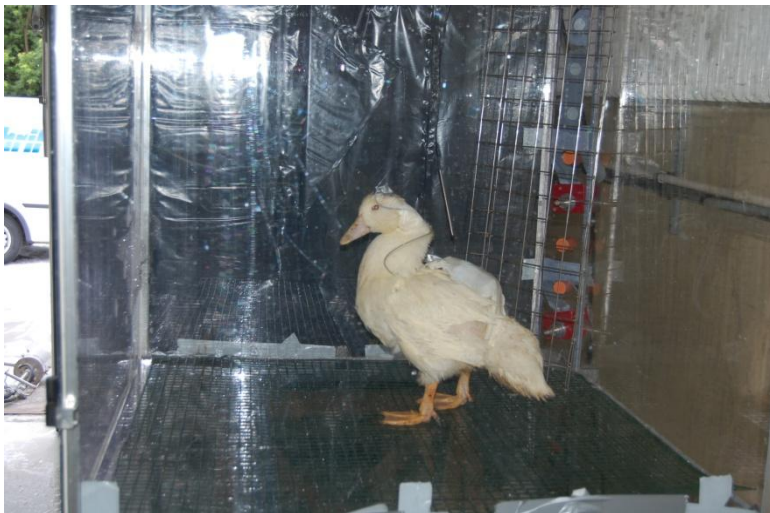
Figure 8: Duck fitted with data logger in lycra harness
