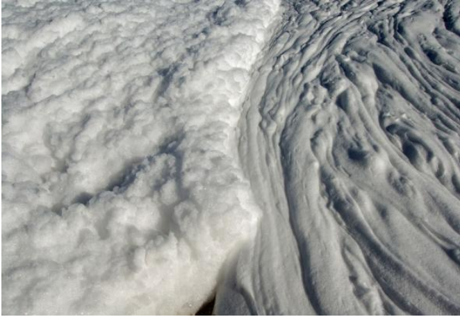
Figure 4 Photographs illustrating the appearance of foam with different expansion ratios
