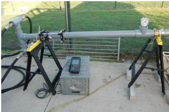
Figure 18 Gas flow meter and improved manifold
