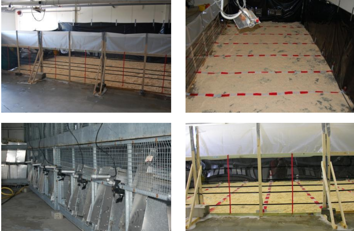
Figure 16 Test pen set up, showing Perspex wall, ariel view and camera positioning
