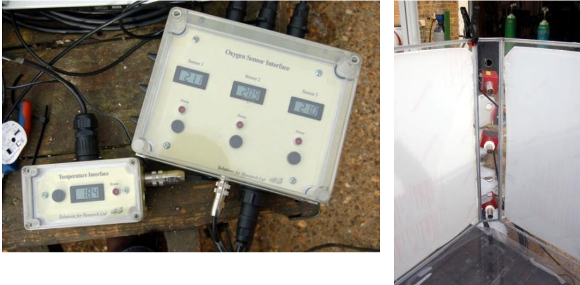
Figure 6: Oxygen sensor interface and positioning in test apparatus
