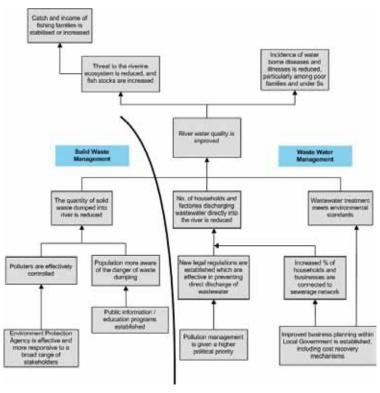
**Figure 6.13** Selecting a strategy from the objectives tree for river water quality (Figure 6.11) by focusing on different sets of objectives. The strategy to the left of the line is a 'solid waste strategy', whilst to the right of the line is a 'wastewater strategy' (source: European Union 2004).2004).
