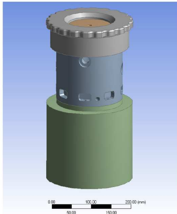
Figure 6 3D sketch of complete assembly, including projector.
