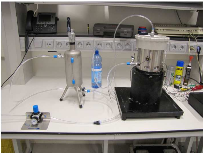
Figure 6 Laboratory test setup: projector and larvae chamber (right), reservoir (middle), pressure regulator (left)
