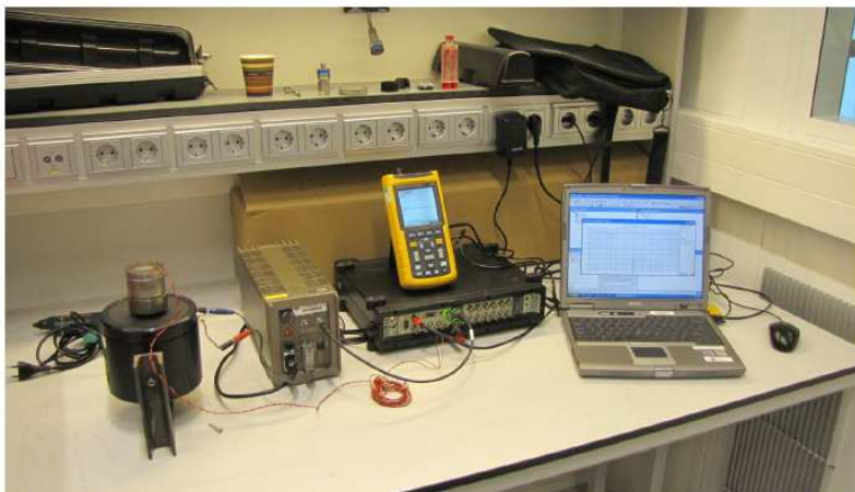
Figure 3 Experimental setup for testing water-resistant accelerometer.
