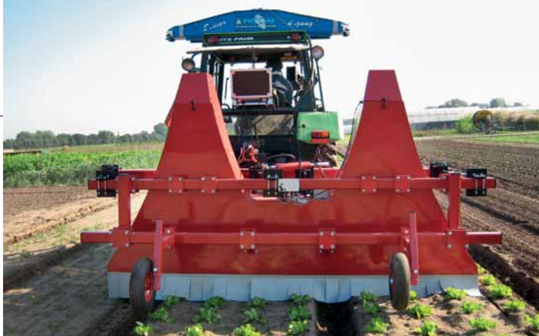
Prototype for recognition and non-chemical control of in-row weeds.
