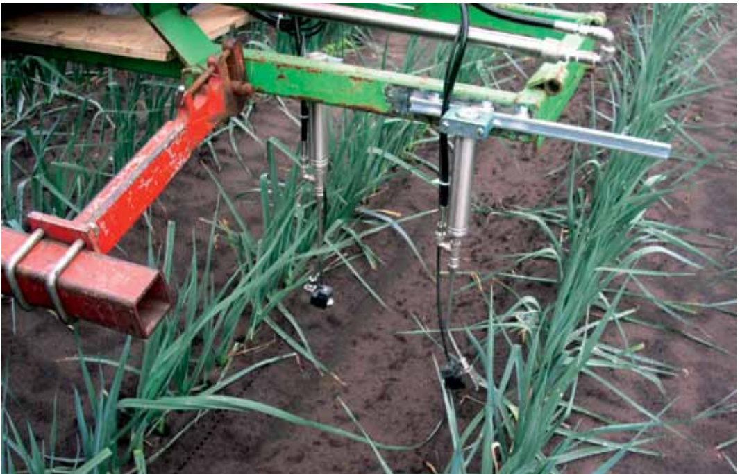
Pulstec is a new fertilisation technique being investigated for injecting fertilisers into the soil under high pressure (50 – 150 bar)
