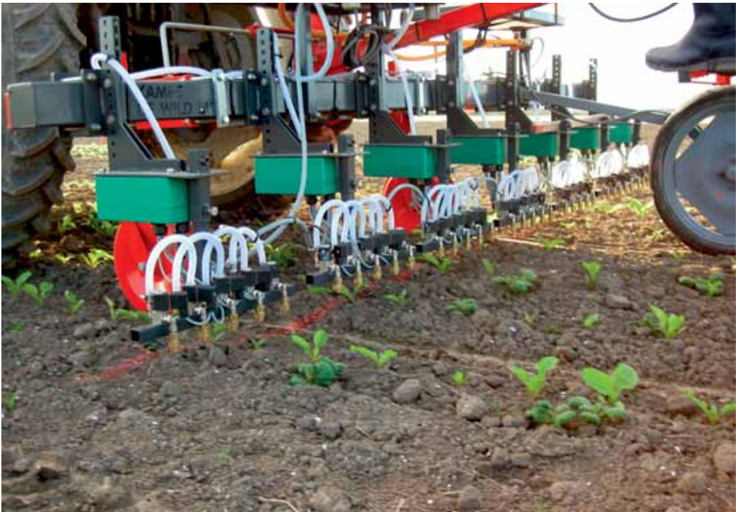
The Weed IT uses fluorescence sensors to control potato volunteers between the sugar beet rows
