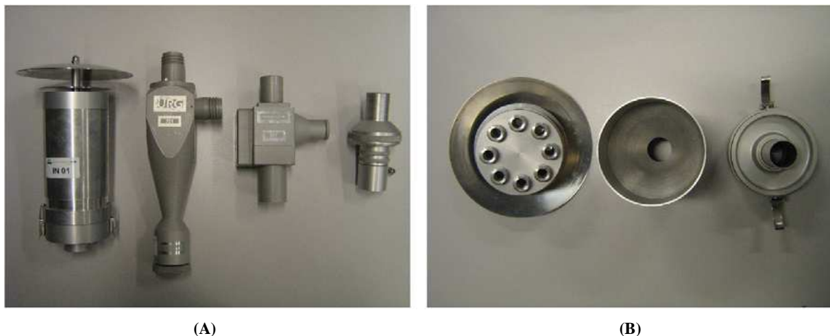
Figure 2. The air inlet head, the PM 10 cyclone pre-separator, the PM 2.5 cyclone pre-separator and the filter holder (A, from left to right), and the construction of the air inlet head (B).
