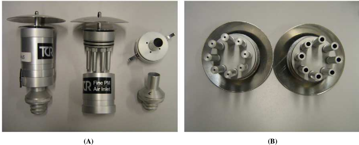
Figure 1. The complete IPS system (A) and the differently sized openings of the impactor nozzles (B) that cause the air above the impaction plate to accelerate (larger openings for PM 10 ; smaller openings for PM 2.5 ).
