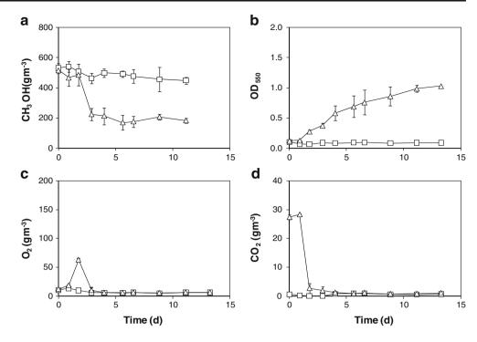
bicarbonate, and an increase in  $OD_{550}$  was measured (Fig. 3a, b). In the absence of bicarbonate, the carbon dioxide concentration gradually increased up to  $13\pm3$  gm<sup>-3</sup> on day 1.8 and was completely depleted by day 2.7 (Fig. 3d). While glucose was present and being degraded, the oxygen concentration remained very low ( $8\pm2$  gm<sup>-3</sup>) and increased up to  $33\pm4$  gm<sup>-3</sup> on day 2.2 of experimenta-
