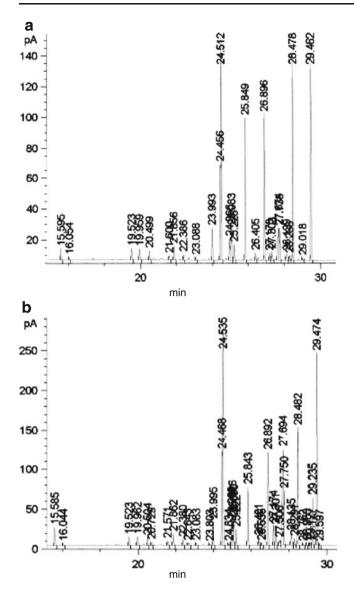
Fig. 5 Fatty acid methyl ester analysis by GC-FID from the  $CH_4$  degrading microalgal bacterial biomass cultivated in the presence (a) and absence (b) of bicarbonate
