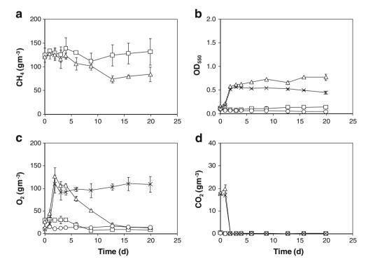
Fig. 2 Time course of methanol (a), biomass (b), oxygen (c) and carbon dioxide (d) concentrations during methanol biodegradation under photosynthetic oxygenation in the absence (*white squares*) and presence (*white squares*) of bicarbonate (5 mM) in tests supplied with AMSM
