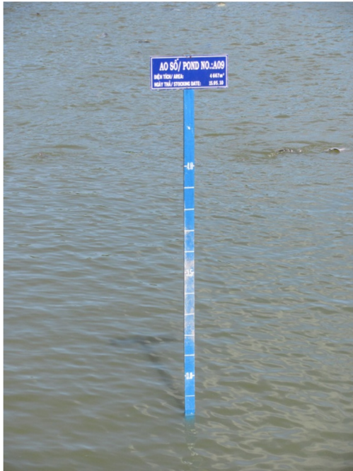
Photo 1. Ruler for recording pond water level changes resulting from draining and filling.
