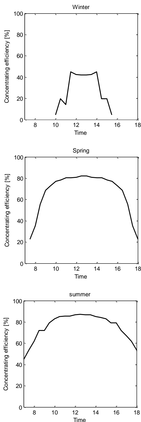
Figure 6: Concentration efficiency of a system with 8 lamellae of 500 mm for a clear day in winter (top), spring (middle) and summer (under).
