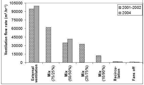
Figure 1. Ventilation flow rate (measured using the internal tracer gas ratio method) during different ventilation situations.
