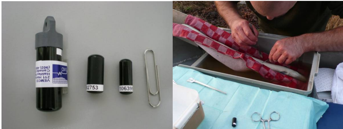
Figure 3 VEMCO transmitters V13 sync-tag, V9 and V7 (left), and a transmitter implanted in an eel (right).
