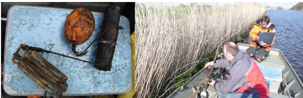
Figure 2 Mooring method (left) and exporting data from a VEMCO VR2W receiver in the field (right).
