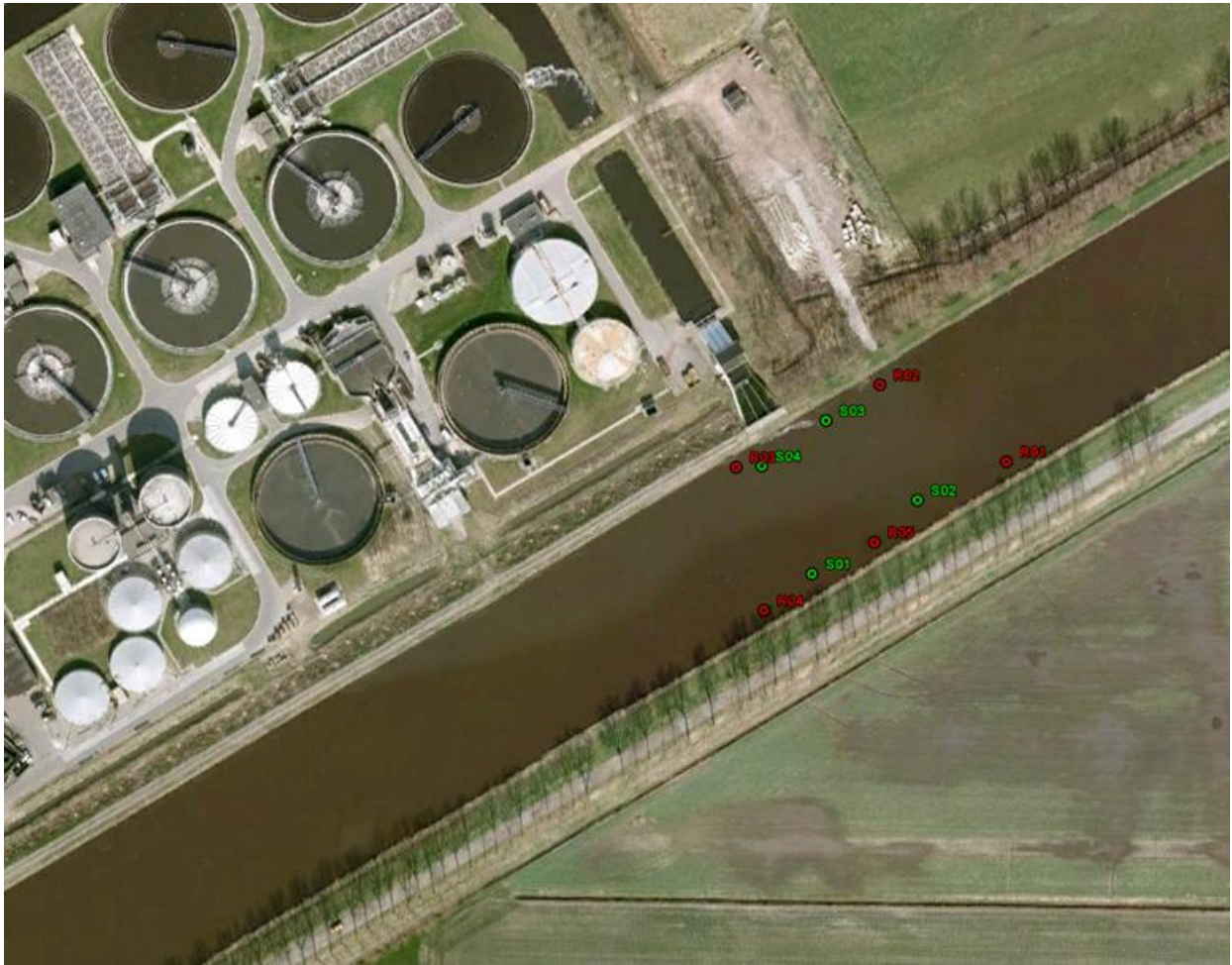
Figure 5 VPS set-up at Groningen in 2009 with 5 VR2W's. Receivers are indicated as red dots, sync-tags as green dots.
