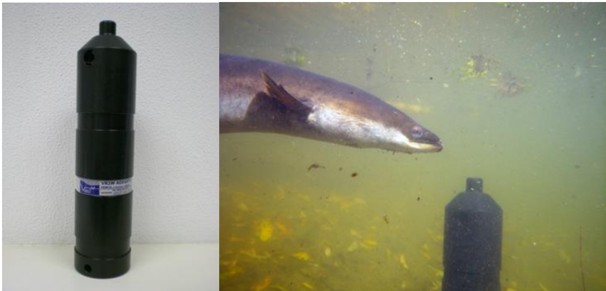
Figure 1 VEMCO VR2W receiver (left) and a receiver under water with a silver eel passing (right).
