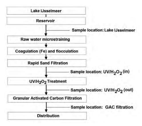
Figure 6.2: Water treatment process scheme of water treatment plant Andijk and sample locations.
