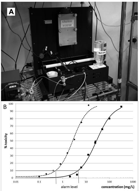
Figure 3.2:A) Picture of the Microlan TOX control and B) the concentration-response curve reflecting the response to increasing concentrations of zinc ( $\blacksquare$ ) and 2,4-dichlorophenol ( $\blacklozenge$ ). Figure 3.2B also presents the alarm limit of zinc at 4.6 mg/L and the alarm limit of 2,4-
