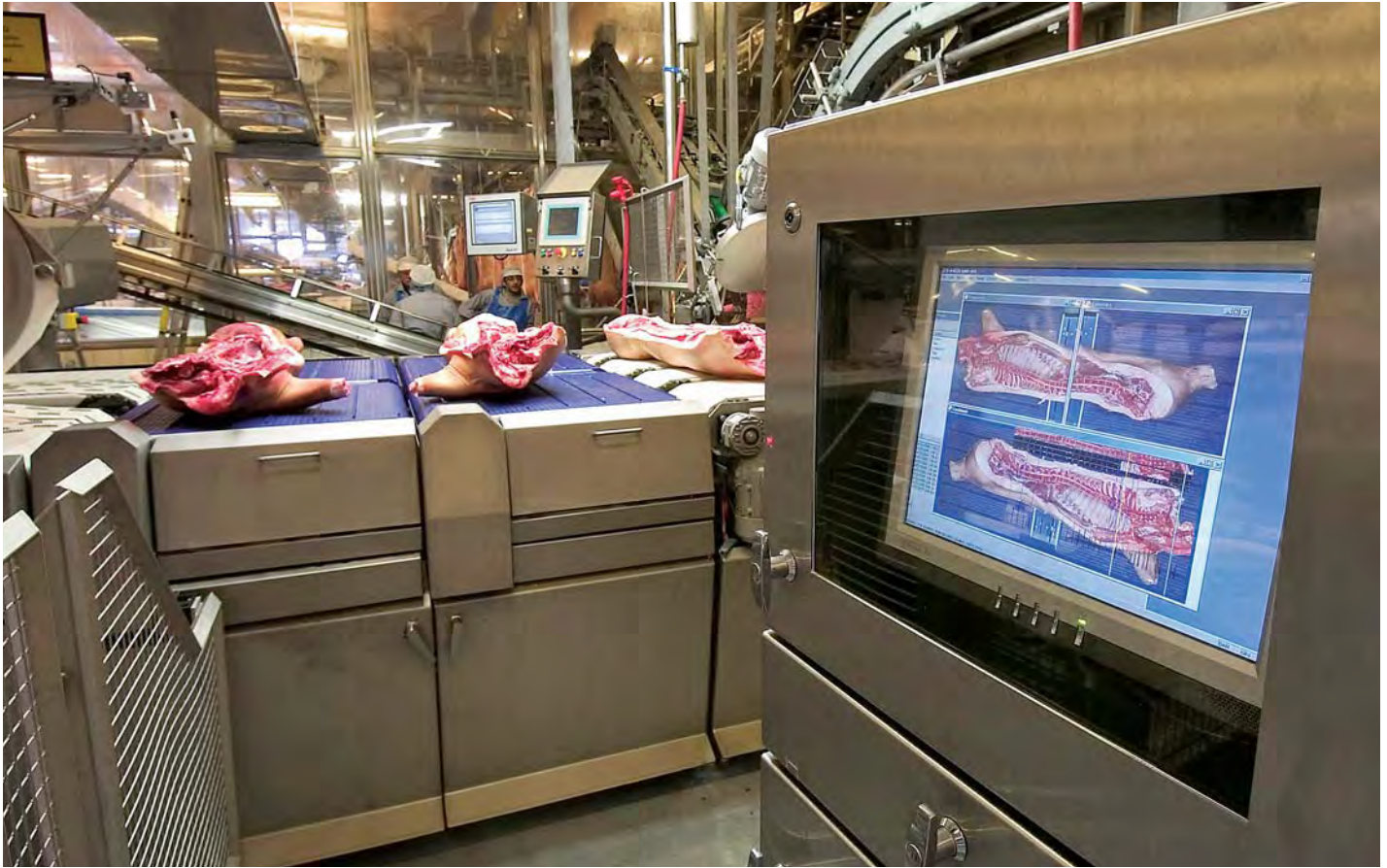
This imaging equipment at Danish Crown determines the most economic points to cut the carcass in order to maximize value
