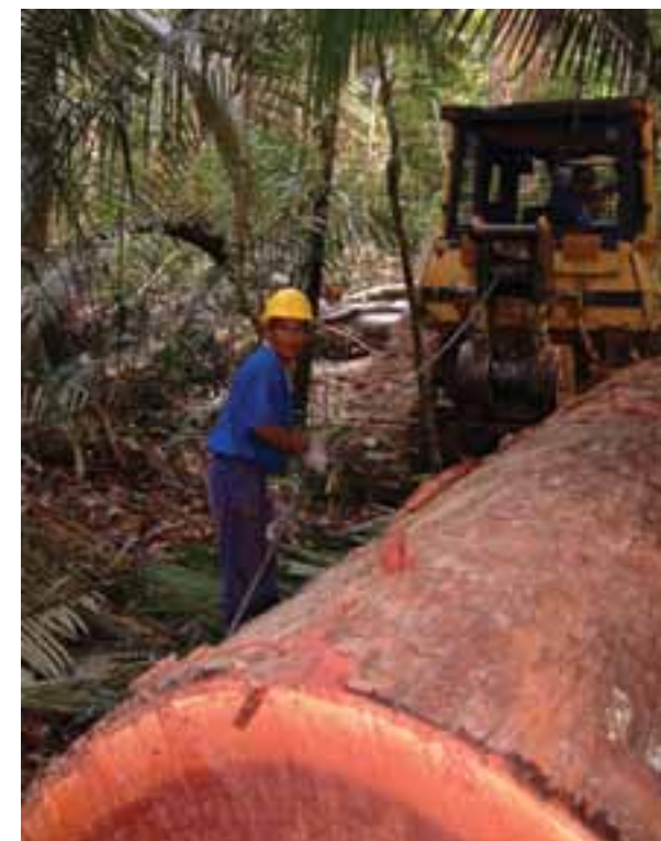
Photo 10.2. Most logs are winched out, over often considerable distances, only lightly disturbing the vegetation, instead of being skidded out behind a tractor from the stump. Here the log has reached the tracked skidder that remains on the skid road. From there a wheeled skidder will take over the load and skid it to the log landing. (Photo N.R. De Graaf)
