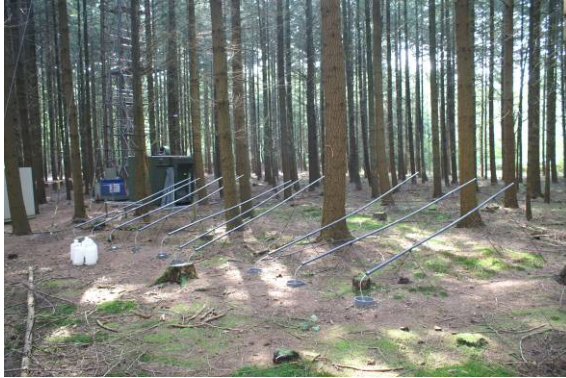
Figure 8 Throughfall samplers at the Speuld site
