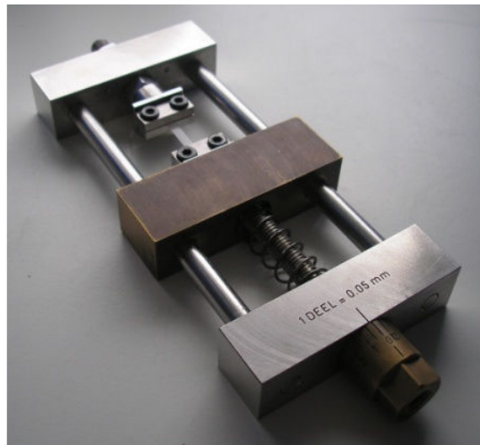
Figure 11: Device for manual loading of SFFT samples. A grid on the screw allows monitoring of the applied elongation.
