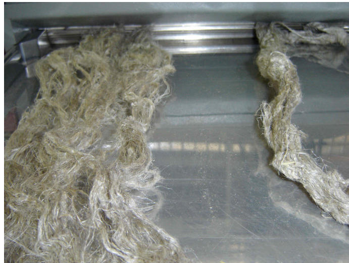
Figure 1: Feeding of fibre samples to Shirley trash separator: fibres oriented parallel to feeding direction with maximum thickness of about 1 mm (left hand sample) and sample with about 5 mm thick fibre clumps (right).
