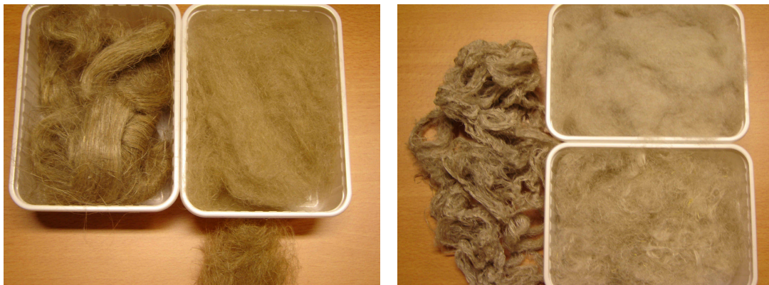
Figure 15: Shirley refined Ekotex flax sliver (left picture) and Ultrasonically treated Ekotex flax fibre coded R1 (right). On each picture: unrefined fibre at left, fine fibre top right and coarse fibre bottom right.
