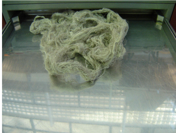
Figure 16: Ultrasonically treated fibre sample R1 after drying, showing fibres glued together in random orientation.
