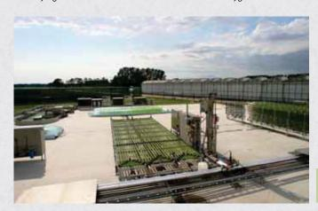
exciting new development. LGem is focusing on the problems that occur when using conventional tubular photobioreactors, including the accumulation of dissolved oxygen and fouling. It has developed a new system which is ten times cheaper than traditional tubular systems.
