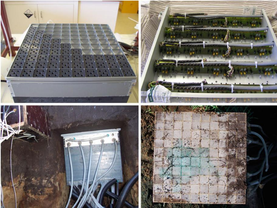
**Fig. 1** Construction details and key features of the multi-compartment sampler (MCS). The instrument has high-spatial resolution with 100 sampling compartments and high temporal resolution of suction, rainfall measurements, and drop counts. To the instrument vacuum is applied which follows ambient suction. The cover of the instrument consists of porous metal plates
