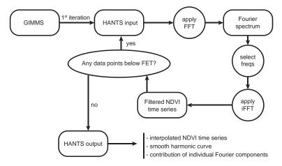
Figure 3.1 Harmonic analysis of NDVI time series flowchart.
