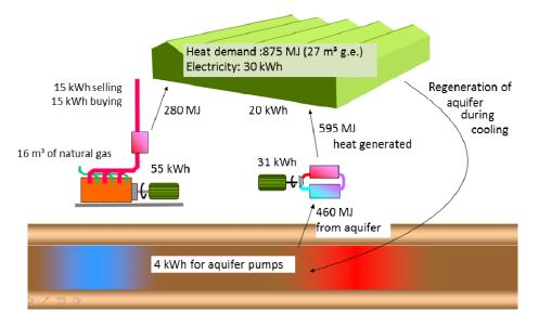
Fig. 3. The energy sources and their use in the concept of the next generation cultivation.
