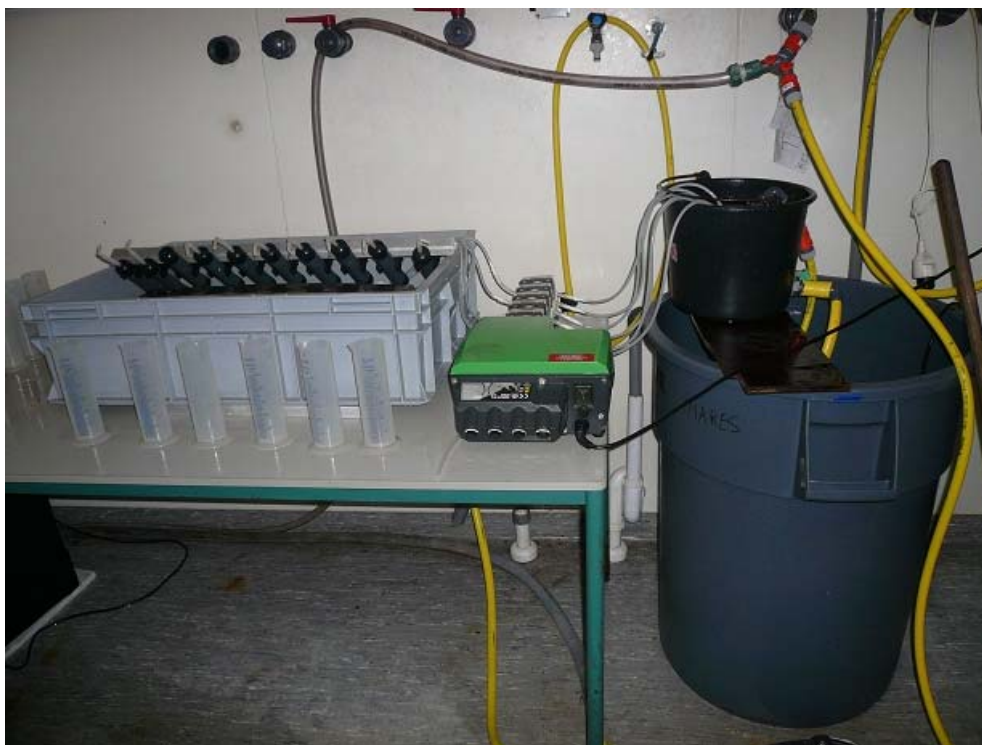
Fig. 3. Set-up to determine filtration rates with tilted cylinders holding Ensis on the left, peristaltic pump in the middle and container holding mixture of silt and algae on the right.
