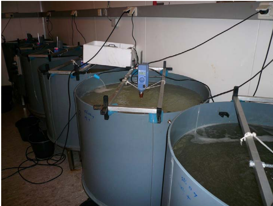
Fig. 4. Circular tanks holding sediment, individually marked Ensis and water. Each container had a different algae and silt mixture. Silt and algae were kept in suspension using an overhead stirrer motor with propeller.
