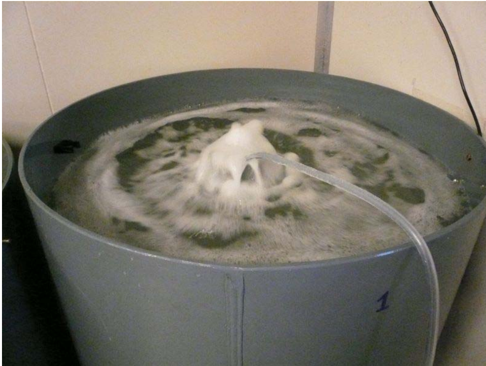
Fig. 5. Test to keep silt suspended with an air pump.
