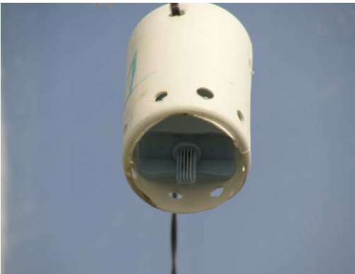
Fig 2.2. Wireless sensor shielded with a ventilated cap. Fig 2.3. The experimental greenhouse equipped with sensors
