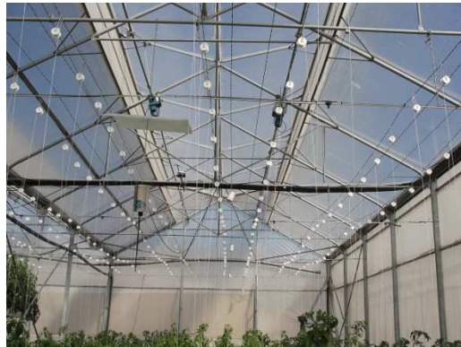
Fig 2.2. Wireless sensor shielded with a ventilated cap. Fig 2.3. The experimental greenhouse equipped with sensors
