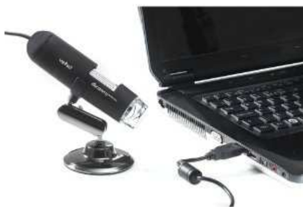
Figure 2.8. A hand-held digital microscope.
