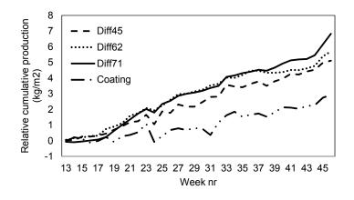
Fig. 2. Cumulative tomato production (kg m<sup>-2</sup>) under diffuse glass (Diff45, Diff62, Diff71) and coated glass relative to the control.
