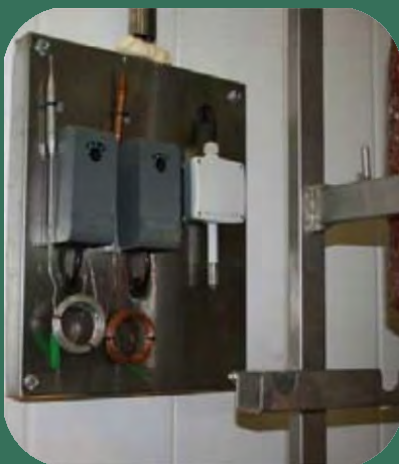
Temperature and relative humidity sensors on the dryer
