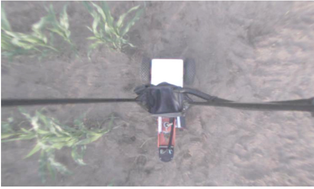
Fig. 6: Clipped image in the headland. The image is ‘wide’ relative to clipped image when the robot is between the rows
