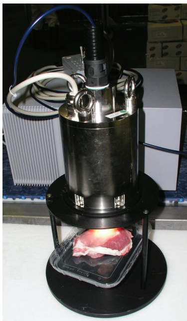
Figure 2. Measurement setup of the contact free probe and NIRS device.
